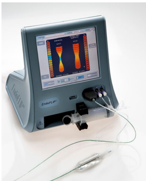
Fig. 1 The functional lumen imaging probe catheter and measurement system. Conductive solution is injected from the syringe into the balloon that surrounds the impedance electrodes and pressure transducers. Cross-sectional area is then calculated and displayed on the screen in real time for a given volume injected and balloon pressure (Image from Crospon Ltd., Galway, Ireland)
